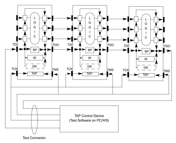
Figure 3. Single Boundary Scan Chain on a Board
