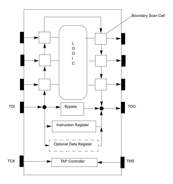
Figure 2. The Boundary Scan Device
